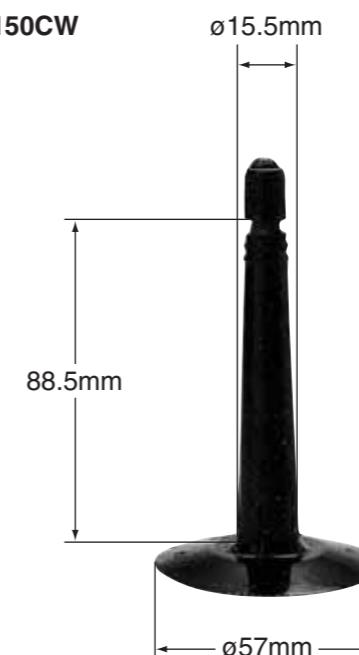
Valves, TR150 and TR150CW, are also called Hand Bendable Valves, that is, their stems are made of very flexible material permitting manual bending in all directions and to any angle.
